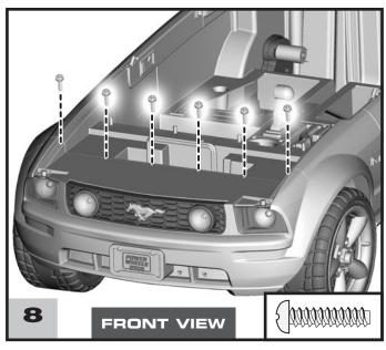
• Insert six #8 x <sup>3</sup>/<sub>4</sub>" screws into the front bumper and tighten.
